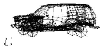
Figure 1: The vehicle finite-element model
