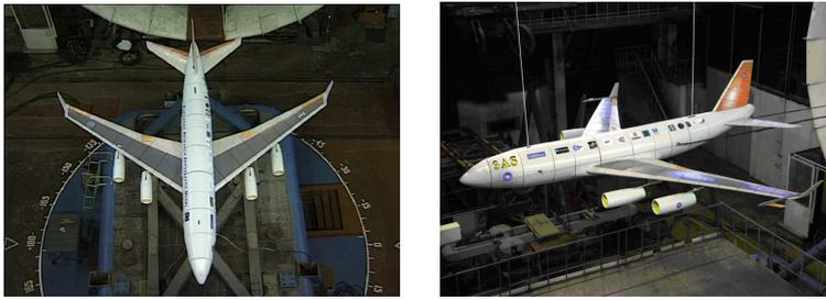
**Figure 7:** Static aeroelasticity test (left) and flutter test on the complete EuRAM (right) in WT T-104.
