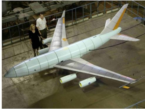
**Figure 1:** The complete EuRAM in TsAGI wind tunnel T-104.
