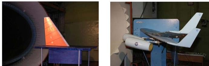
**Figure 6:** Forward aileron (left) and inner aileron with flexible SDS (right).
