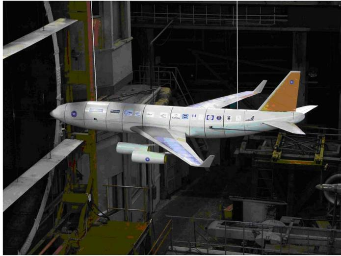
**Figure 8:** Gust response test on on the EuRAM .
