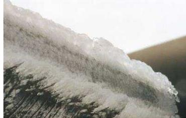
**Figure 4:** Severe mixed ice accumulation on the tail of a full-scale NASA test aircraft [10].
